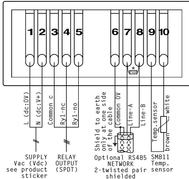
**RS 485 NETWORK CONNECTIONS 2-twisted pair shielded cable:**
